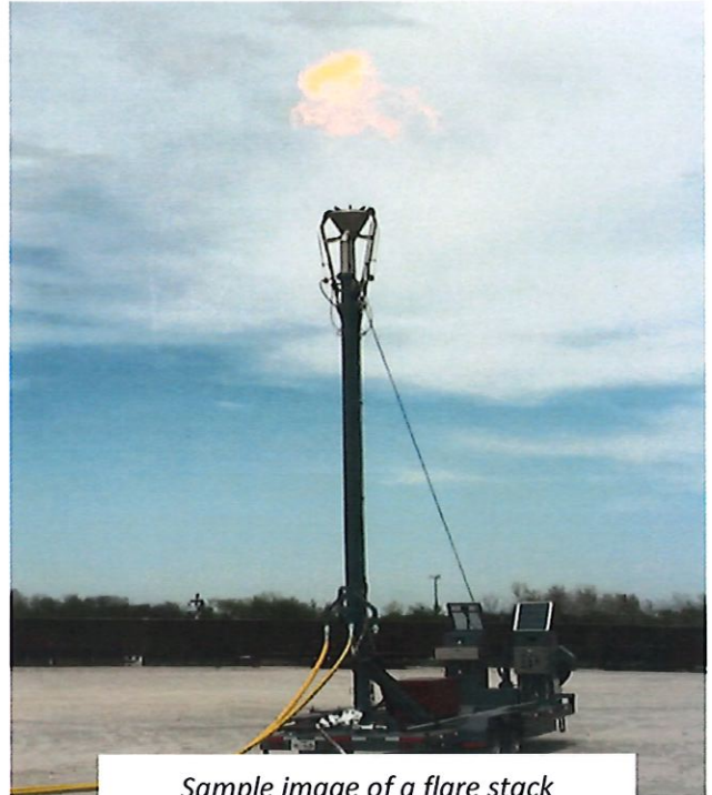
Sample image of a flare stack
